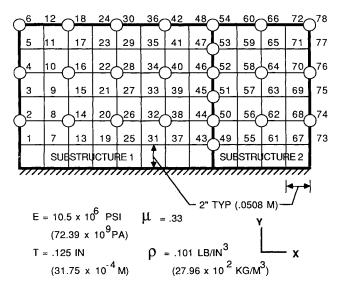
Fig. 1 Rectangular cantilever plate.
